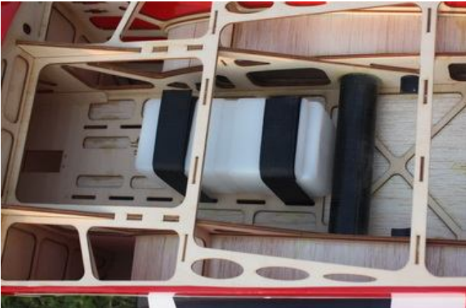
Pre-assembled and mounted gas tank
