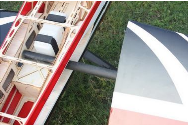
Increased diameter carbon fiber wing tube over previous versions
