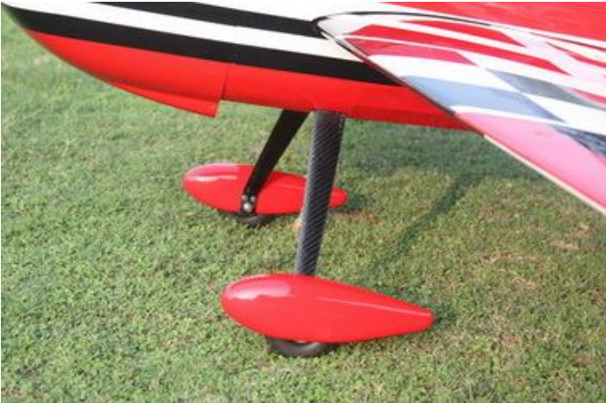
One piece air foiled carbon fiber landing gear
