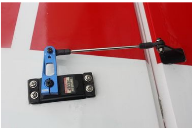
26mm/1in for aileron No. KAG0S70F/KAG0S70H/KAG0S70J
