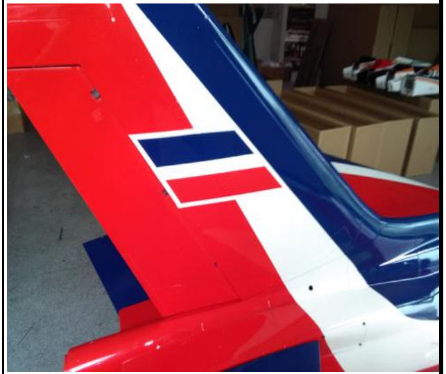
48. The picture after the vertical fin assembled.
