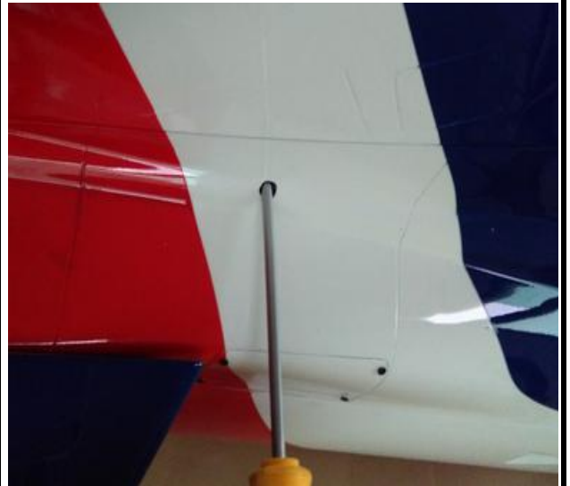
47. Lock the vertical fin with screw.
